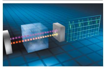
Many gases absorb infrared light at certain wavelengths. The absorption spectrum is distinctive for each gas in question. Infrared Open Path and the Point Technology from MSA use electronically-modulated IR radiation sources at two different wavelengths. One wavelength is typical for the gas to be measured, while there is no infrared absorption by atmospheric gases for the other wavelength.
