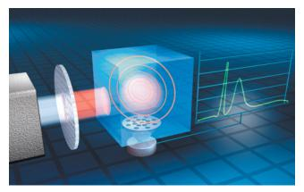
Photo-acoustic sensor technology was developed by MSA for the detection of toxic or combustible gases at very low concentrations. A gas sample is introduced into the measurement chamber and the sample is exposed to a specific wavelength of pulsed infrared light. If the sample contains the gas in question, it will absorb an amount of infrared light proportional to the concentration of gas present.
